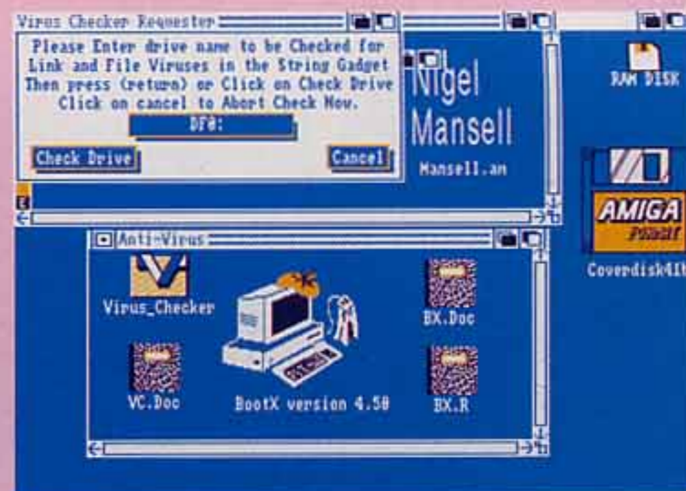
When you select the Link/File Scan option, you'll be asked to tell the program which drive the disk you want scanned is in. Type the name (for example, df0: for the internal drive) then click on 'Check drive'.
